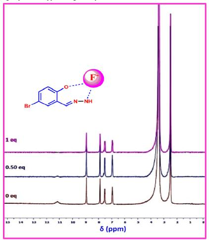
Figure 8 <sup>1</sup>H NMR titration of BHP with  $F^-$  (0-1 equiv) in DMSO- $d_6$
